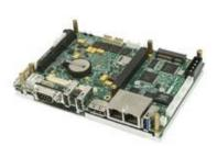
The module contains: CFast connector, two Ethernet channels, 7x USB ports, 1x Serial ATA port, 8x serial ports, NAND Flash drive. Module's functionalities can be extended by connecting additional modules in StackPC, <u>StackPC-PCI</u>, PCI-104, PCIe/104, PCI/104- Express format.
